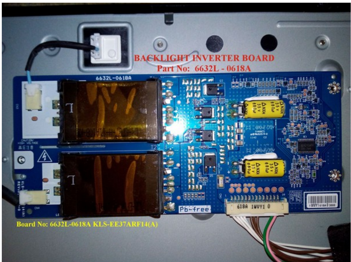
Bild. 8 (Backlight Inverter Board: 6632L-0618A)
