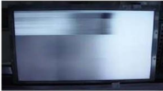
Horizontal Block Gate TAB IC Defect
