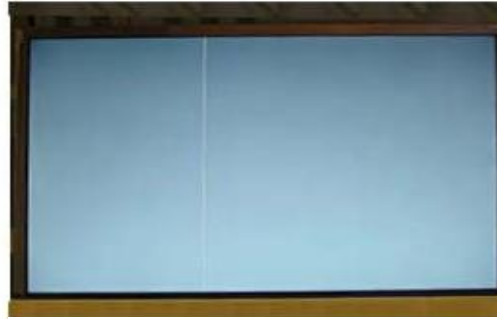
Vertical Line Source TAB IC Defect
