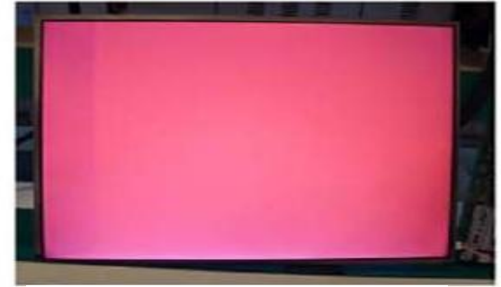
Vertical Block Source TAB IC Defect
