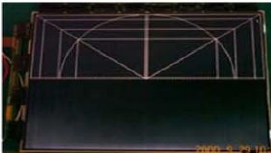
Horizontal Block Gate TAB IC Defect
