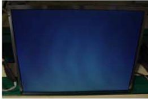
Panel Mura, Light leakage
