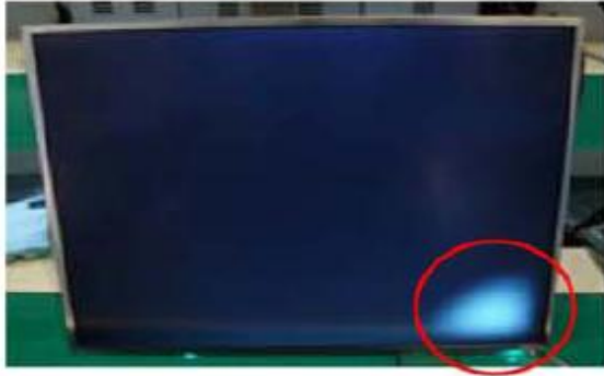
Panel Mura, Light leakage
