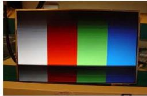
Horizontal Block Gate TAB IC Defect
