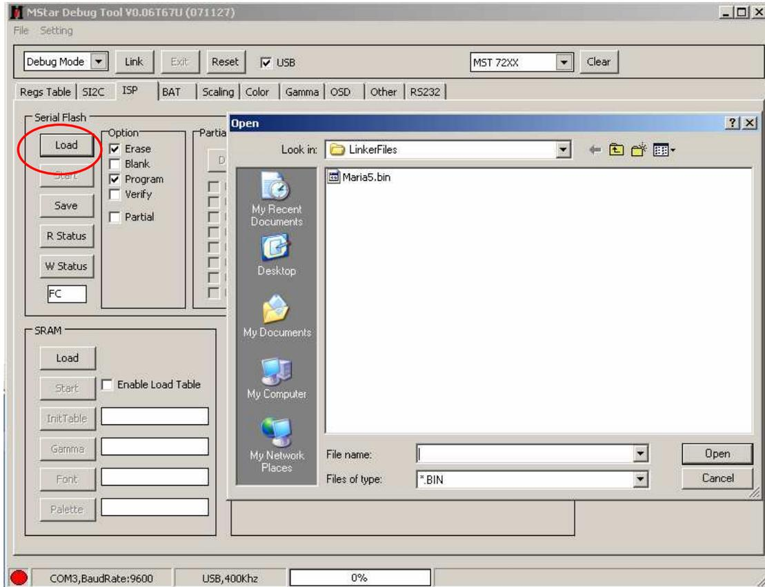
When the software is loading, bar on the bottom is proceed. (Below picture) When it is reached on % 100, the software loading process is complete.
