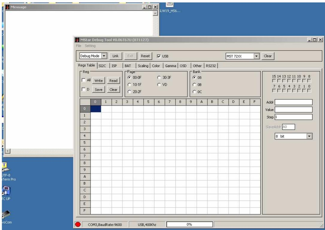
You do not need any arrangement on interface, but you can control Uart port number and bound rate (which bound rate must be 9600 for SM/U1/SH/DH chassis) with Setting menu. For Setting Menu you must press “Settings” tabs.
